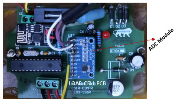
Figure 8. (a) Top view of the convergence circuit, (b) Bottom view of convergence circuit, (c) printed circuit board of the strata monitoring device. 15
