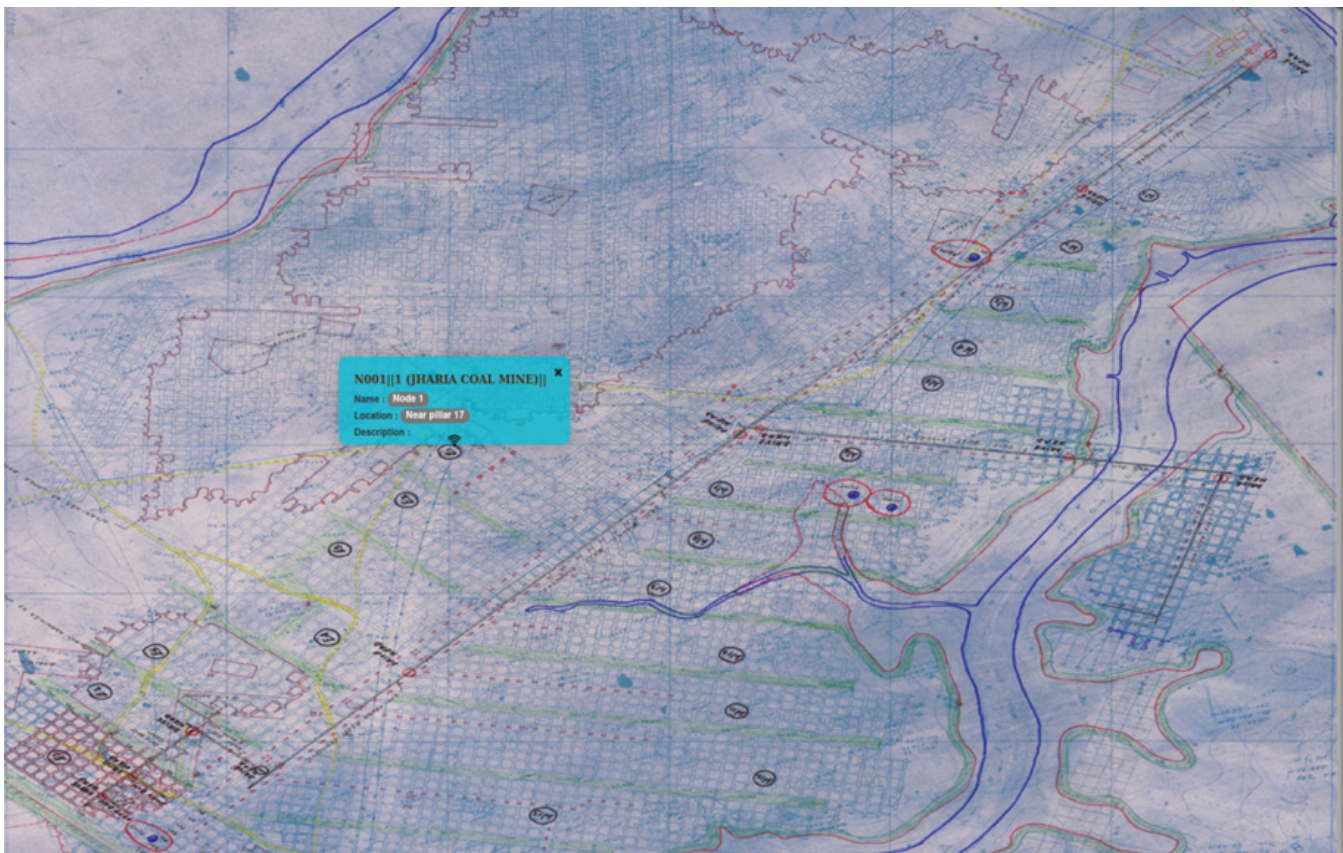
Figure 13. Incorporation of wireless nodes at designated locations on the mine map.
