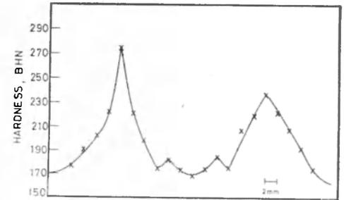
Fig 5. Variation of hardness across the welded section.
