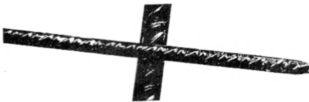
Fig. 7. Tensile test. Fracture outside the weld
