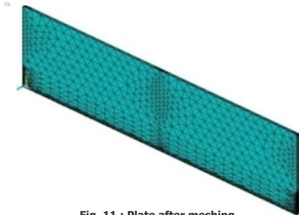
Fig. 11 : Plate after meshing
