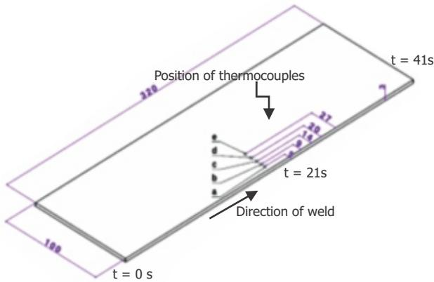
**Fig. 2 : Geometry of plate with position of thermocouples.**
