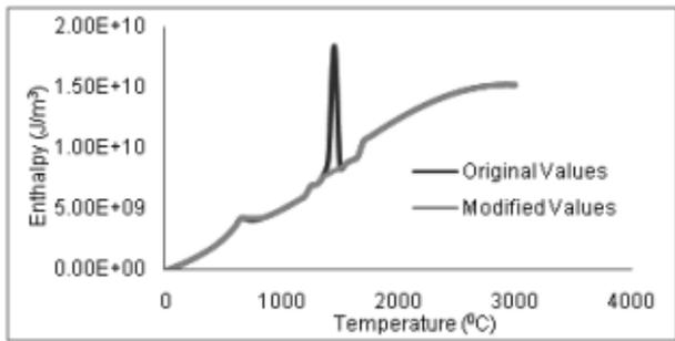
**Fig. 7 : Variation of calculated and modified values of enthalpy of AISI 430.**
