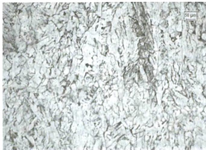
Figure 3. (Sample A) Weld prepared in SAW process with 10% slag-mix
