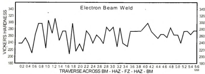
**Graph G2 :** Micro Hardness Traverse for Welds made in Solution Treated Plates
