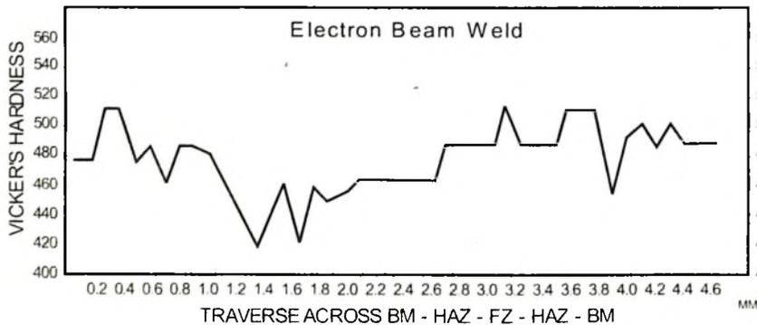
**Graph G3 :** Micro Hardness Traverse for Welds made in Solution Treated Plates & given Post Weld Ageing Treatment.
