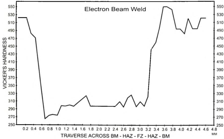
**Graph G1 :** Micro Hardness Traverse for Welds made in Aged Plates.
