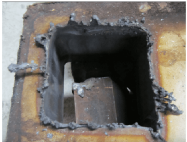
Stainless Steel dross is difficult to remove
