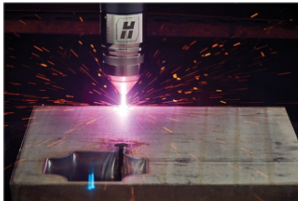
Stainless Steel cutting chart 105 A with Air Hypertherm Powermax105® plasma cutting system
