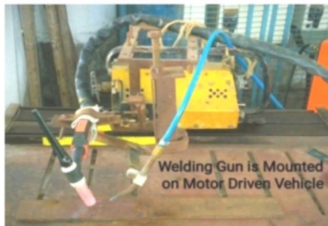
Fig. 1 : GTAW welding gun mounted on motor driven vehicle
