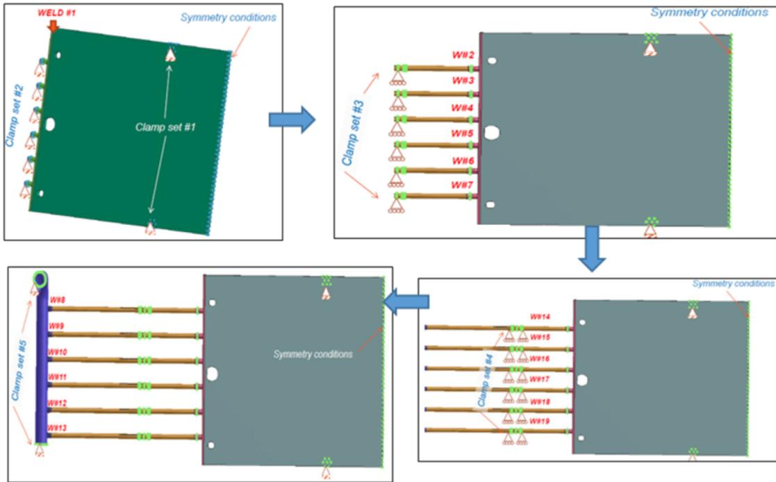
Fig. 4 : Clamping details with welding sequence for configuration 1
