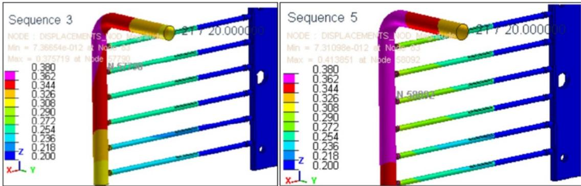
Fig. 7 : Welding distortion for welding sequence 3 and 5 for configuration 1
