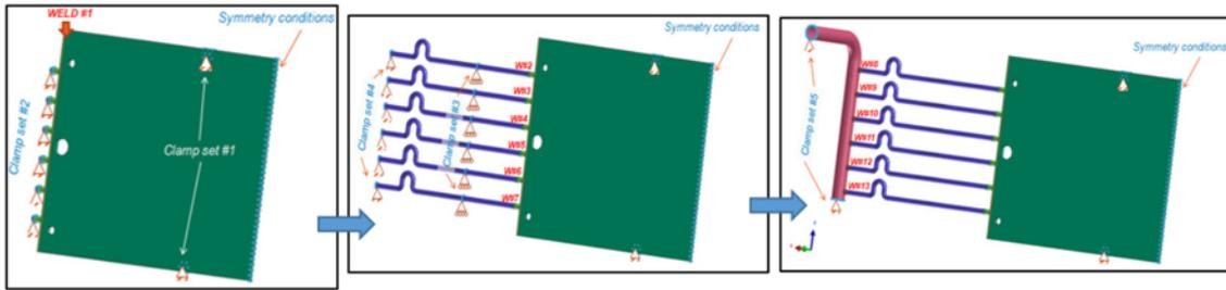
Fig. 6 : Clamping details with welding sequence for configuration 2
