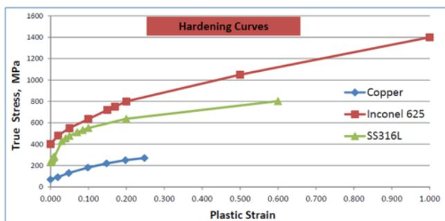
Fig. 3 : Straining Hardening curve for the materials
