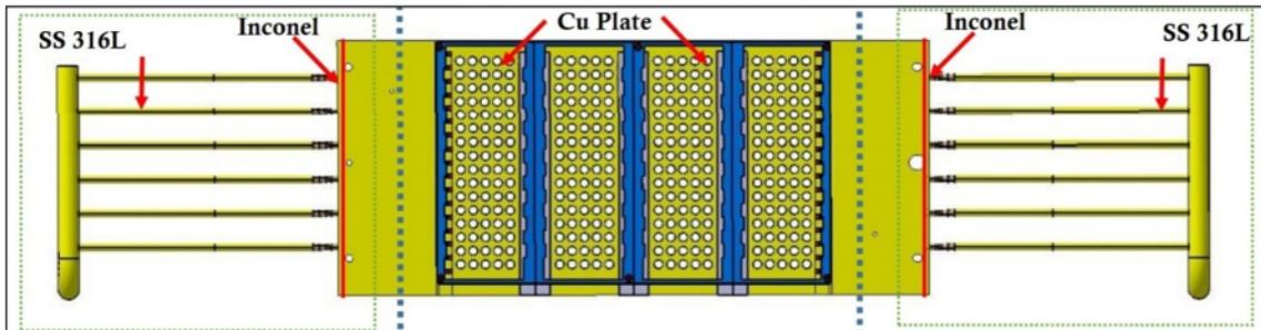
Fig. 1 : Beam Source Grid with the Hydraulic connections
