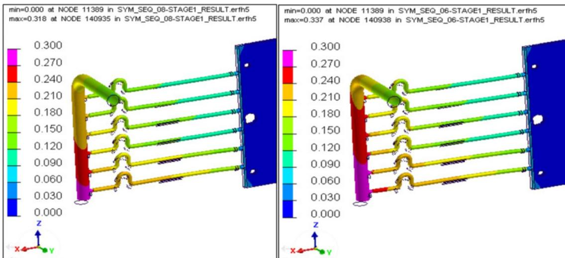
Fig. 8 : Welding distortion for welding sequence 7 and 5 for configuration 2
