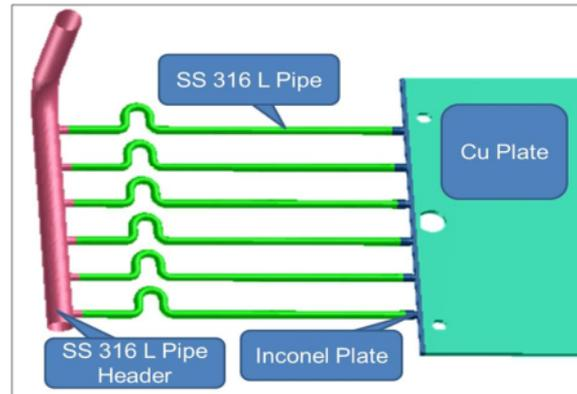
Fig. 2b : Modified design with U-Bend
