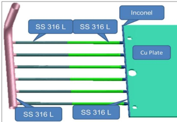
Fig. 2a : Baseline design of Hydraulic pipe welded with copper grid;
