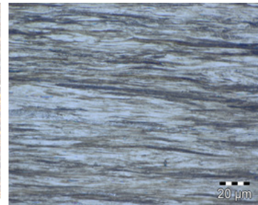
Figure 3(c). Fine pearlite & ferrite in longitudinal direction at 1000x
