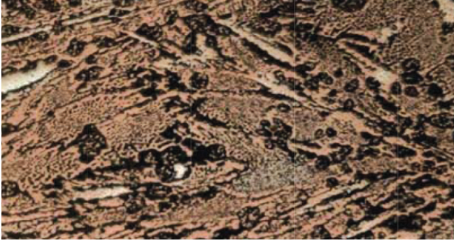
Fig.7 Model of the structure of white cast iron at the forming ratio (60%)
