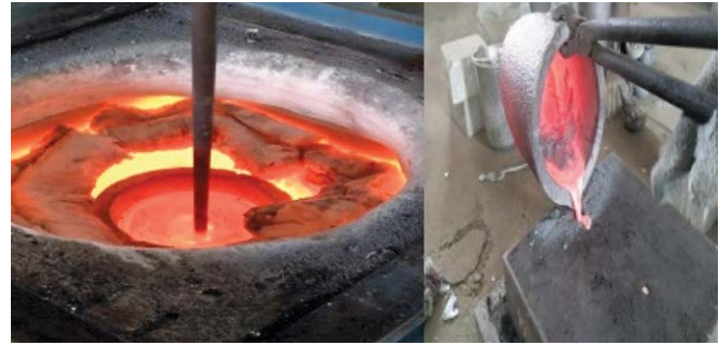
Fig.5: Stir casting process
