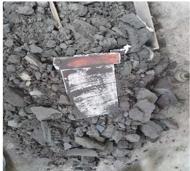
Fig.6: Copper chill and composite after casting
