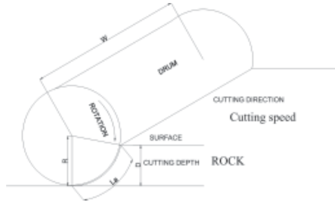
Fig.4 Length of arc of drum in contact with the rock during cutting operation
