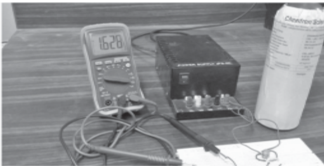
Fig.4 Laboratory set up for TGS2611 methane sensor
