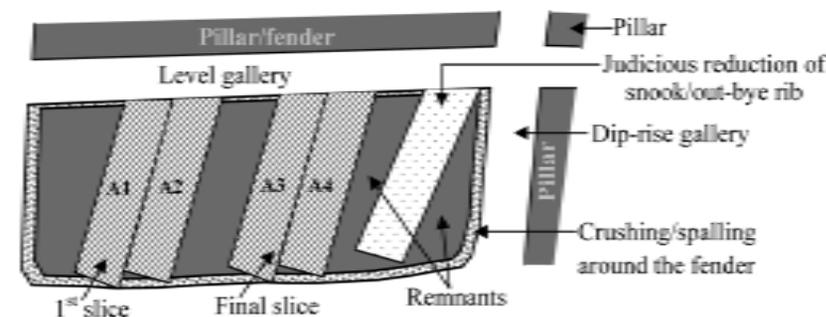
Fig.11 Reduction of a snook through a central cut in the snook during the mechanized depillaring
