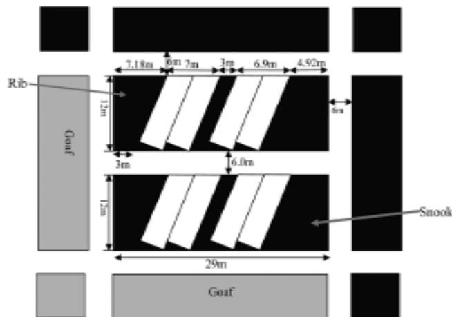
Fig.3 Positions of rib and snook for a typical manner of extraction of a pillar during mechanised depillaring
