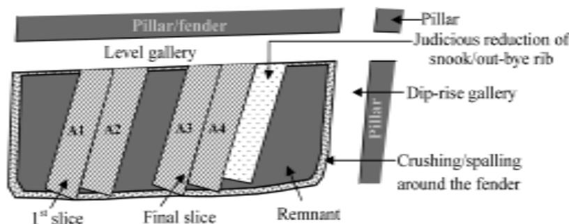
Fig.10 Reduction of a snook along existing slice side during the mechanized depillaring
