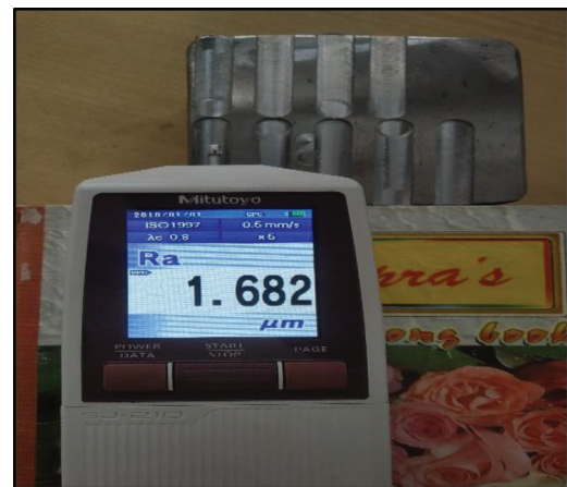
Figure 2. Measurement of surface roughness using Talysurf instrument.
