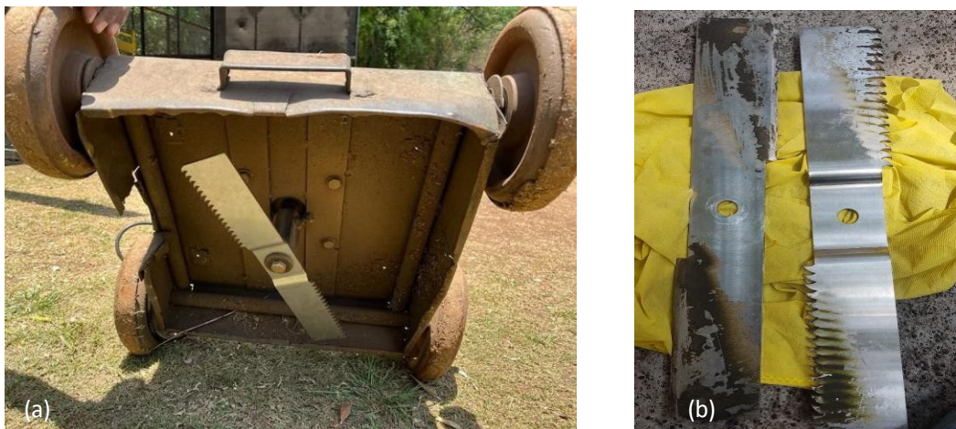
Figure 18. (a) Field testing of bionic blade Lawnmower Cutter (b) Plain blade vs Bionic blade (SS 304) Lawnmower cutter
