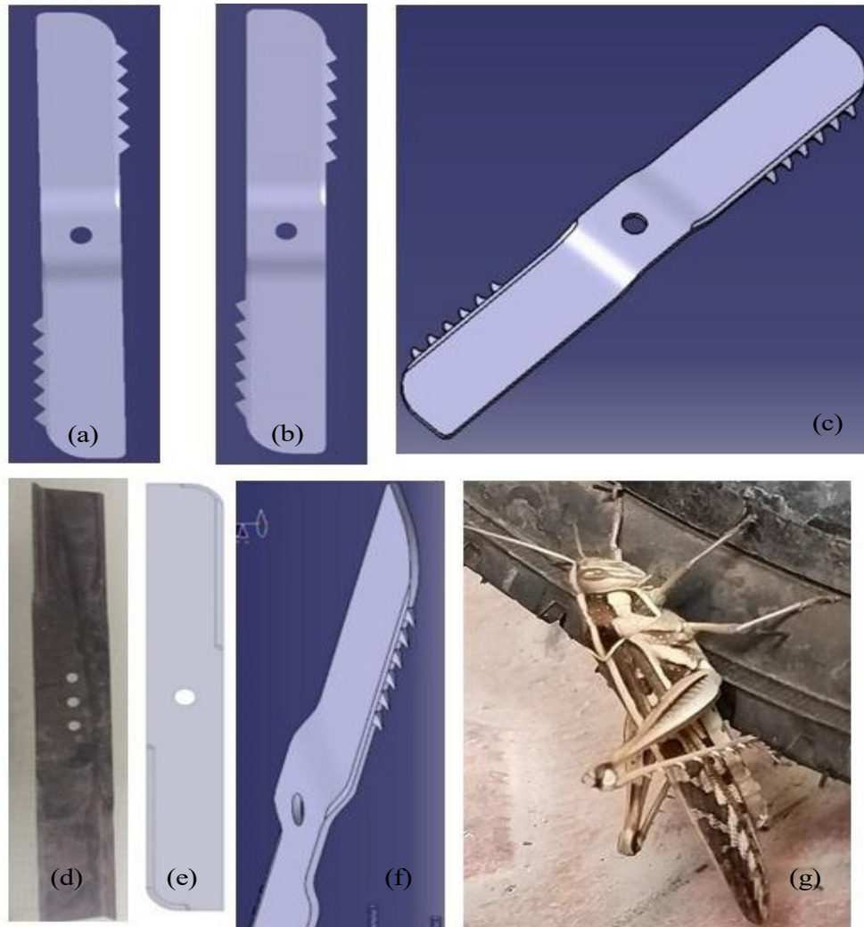
Figure 3. Bioinspired lawnmower cutter blade (a) 45°-45°, (b) 30°-60° tooth angle (c) Bionic blade isometric. (d) Plain blade conventional (e) Plain blade rounded edge (f) Bionic blade (g) Grasshopper serrated leg.
