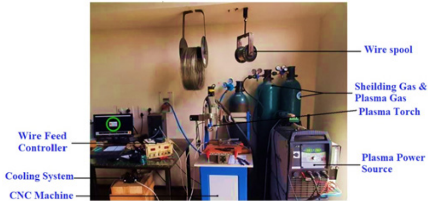
Figure 2. Experimental setup for plasma remelting.
