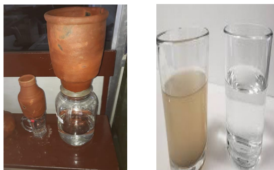
Figure 4. Indigenous porous clay pot with filter disc to remove mud in water.
