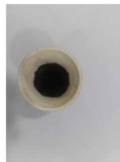
Figure 1. Graphene Sand Composite in crucible.
