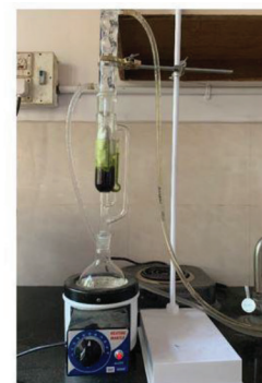
Soxhlet extraction of Syzygium jambos leaves using ethanol
