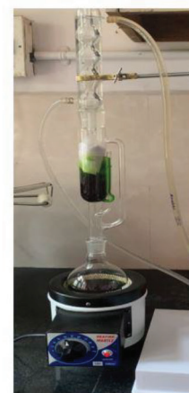
Soxhlet extraction of Psidium guajava leaves using ethanol
