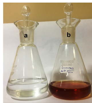
Figure 1. Green synthesis of AgNPs using Chaetomorpha antennina extract: (a) Control (b) Silver nanoparticles synthesized using CA.
